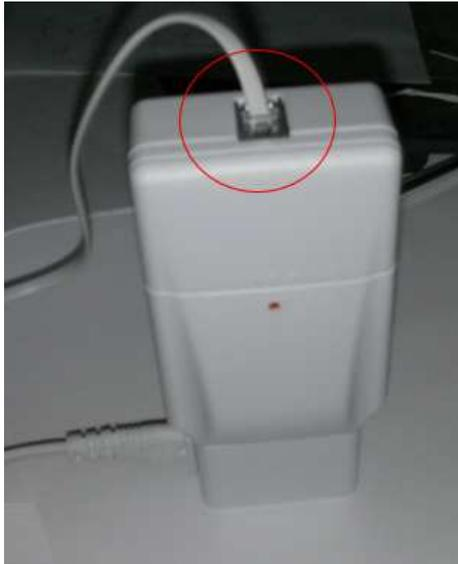
You don't need to enroll or set up the X10MU – just connect it to the Visonic Alarm and to the mains.
