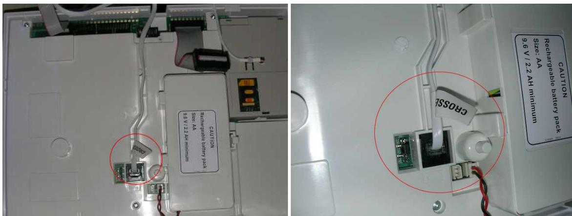
Above: Crossed RJ11 cable connected to the Visonic panel
